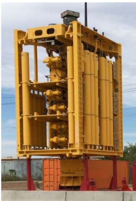
Figura 2.17 – Lower Marine Riser Package (LMRP) [21]
