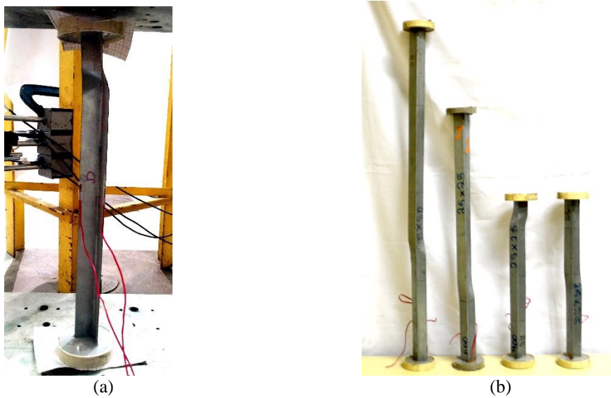
Figure 3.16: (a) Close view of the most deformed region of specimen 25t0.8 L400 just after collapse and (b) joint view of the specimens belonging to the 25t0.80 series after the load removal.
