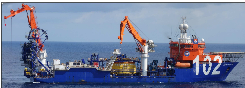
Figura 2.9 – North Ocean 102 (McDermott) – Método Reel-Lay com carretel horizontal.
