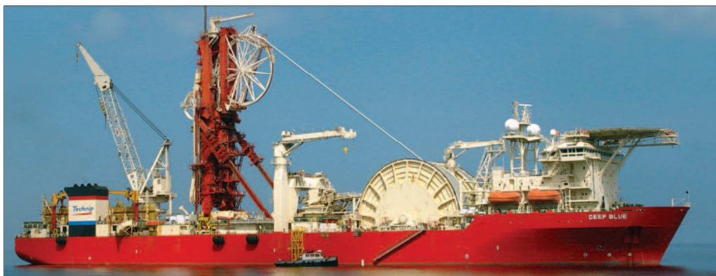
Figura 2.11 – PLSV Deep Blue (Technip) – Método vertical Reel-Lay com moonpool .
