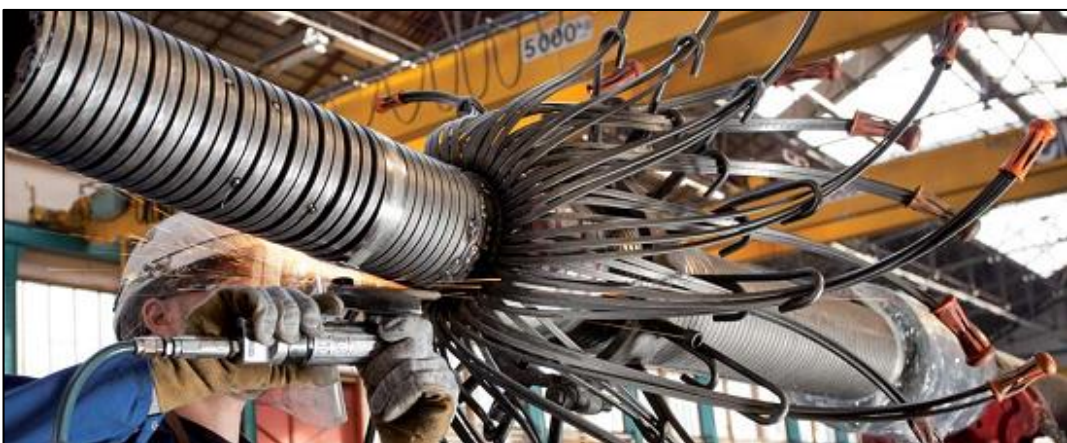
Figure 15. End-fitting mounting - folding process (TECHNIP, 2015).
