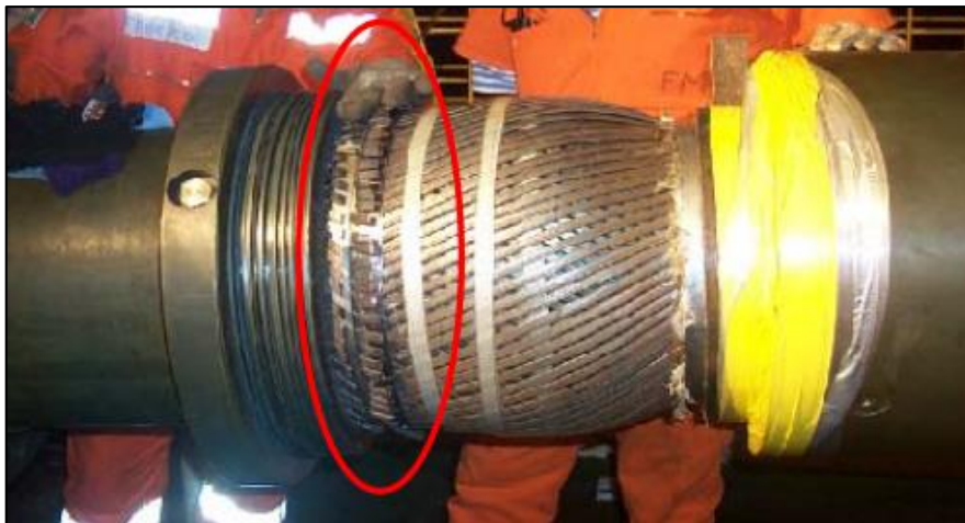
Figure 19. Anchoring and alignment of the tensile armor wires inside the EF (DAFLON, 2010).
