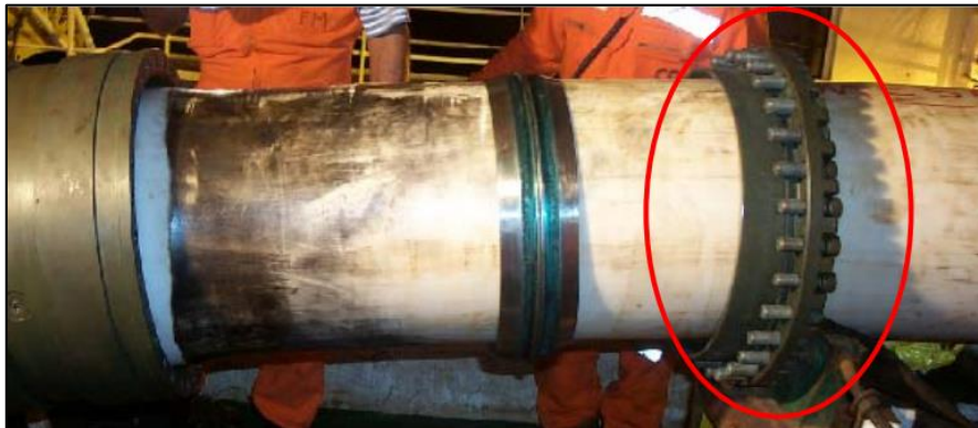
Figure 20. Fastening the rear flange of the EF (DAFLON, 2010).
