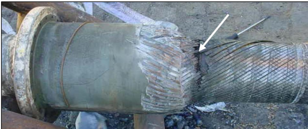
Figure 3. Armor wire failure in the EF (MARINHO et al. , 2007).
