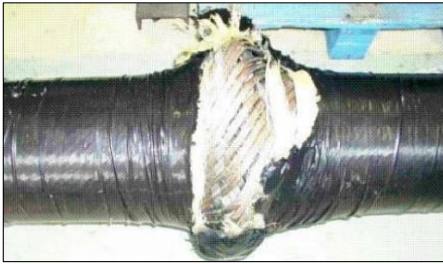
Figure 11. Flexible pipe with birdcage (BECTARTE et al. , 2004).
