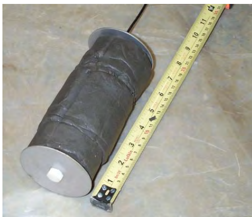
Figura 2.10: Soil compression gauge envolto pelo solo (WEINMANN et al. , 2014)
