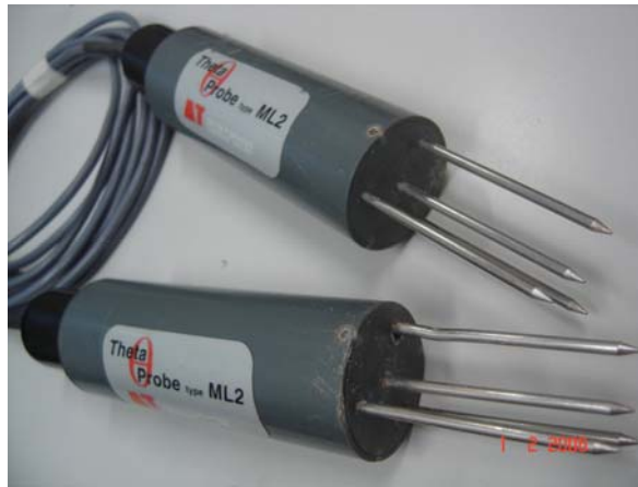
Figura 4.3 – TDR (Delta – T Devices, UK, 2000)
